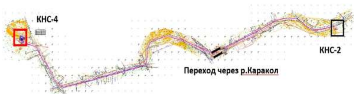
Figure 4. Layout of designed sewerage collector
