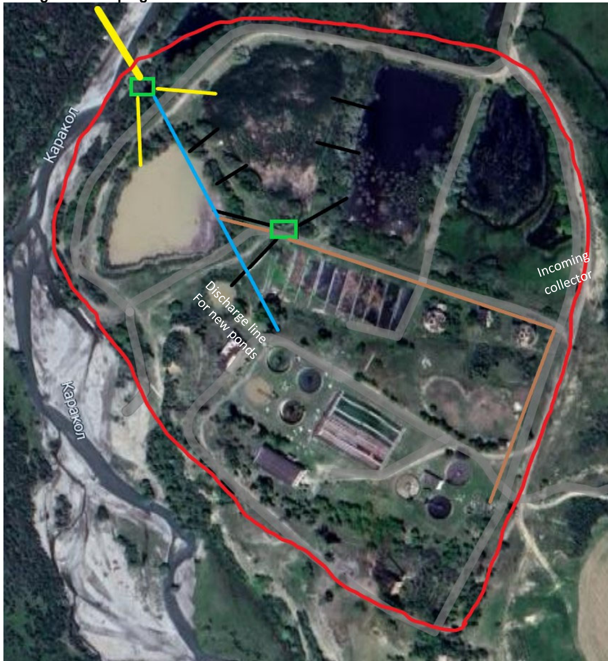
Figure 5-4. Piping Details of Karakol WWTP Ponds
