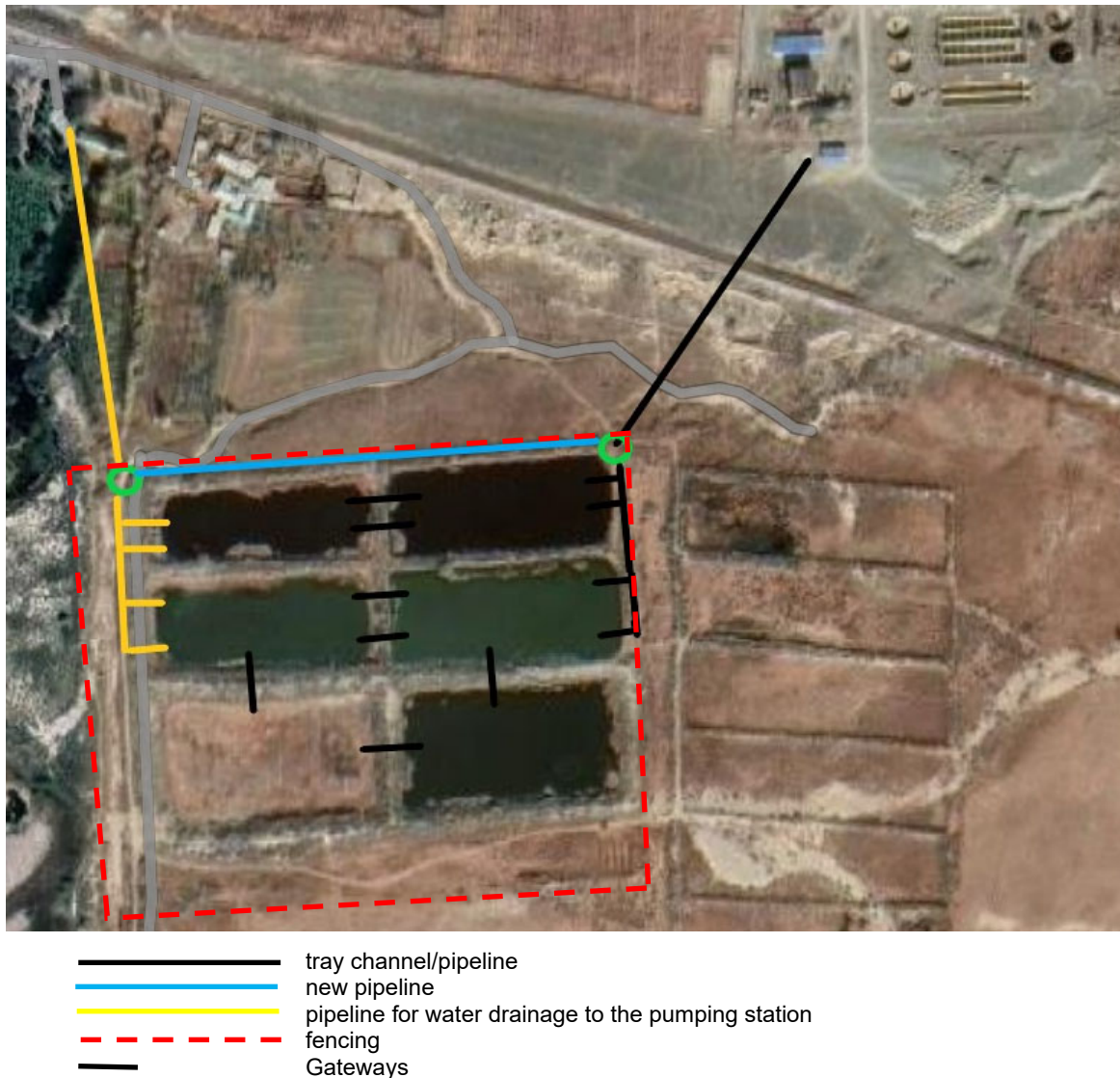
Figure 5-2. Piping Details of Balykchy WWTP Ponds
