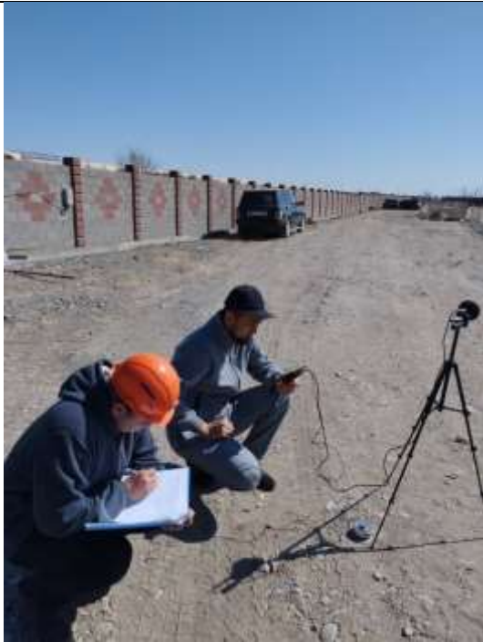
Noise monitoring has been conducted at Balykchy WWTP site
