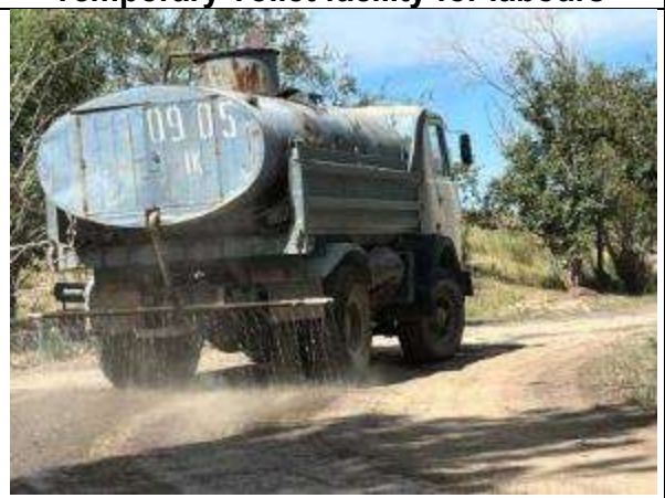
Water sprinkling for dust emission control
