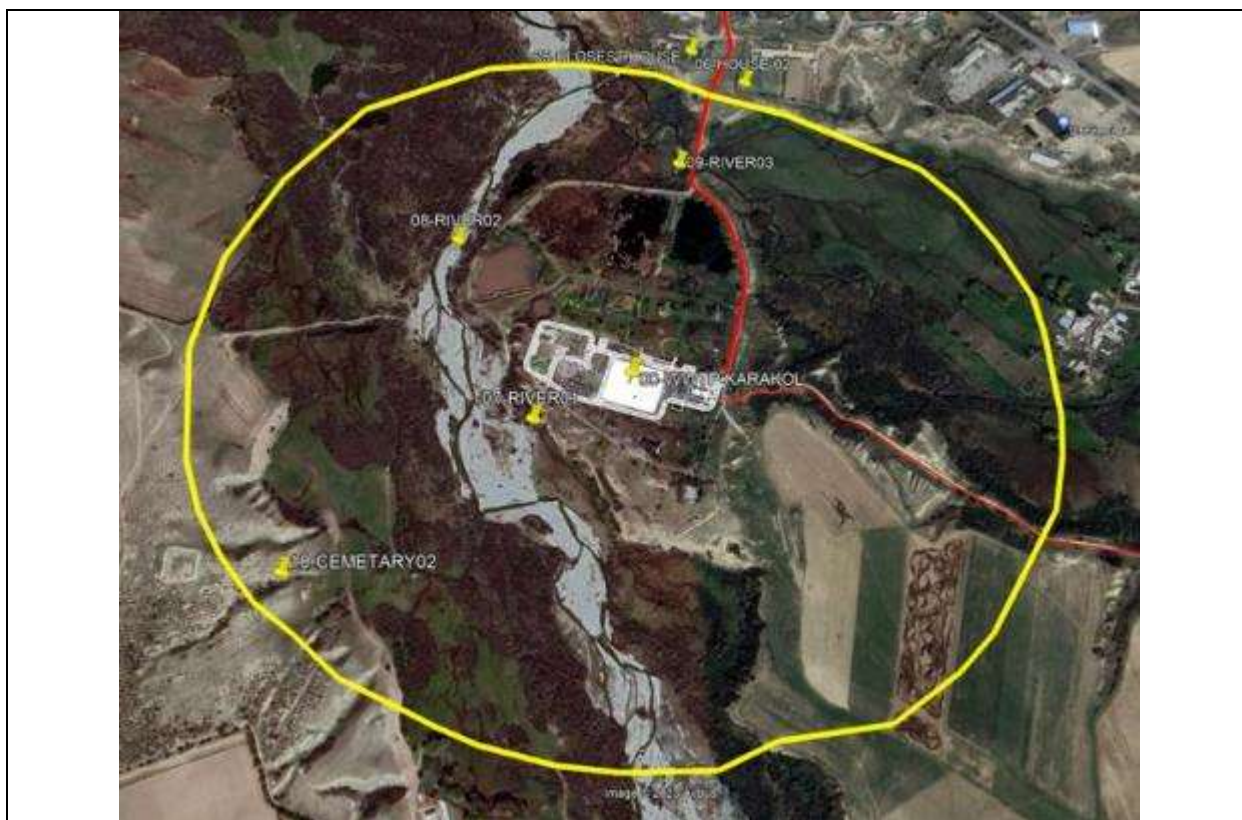
Figure 4-2: Sanitary Protection Zone of the sewage treatment plant 400 metres (Yellow contour is the SPZ boundary of the WWTP. The size of the SPZ is 400 metres from the boundary of the WWTP)
