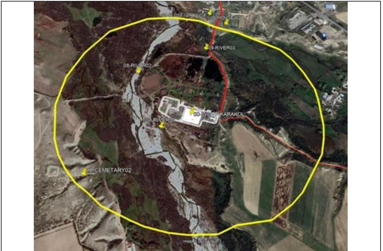
Figure 5-1: Sanitary Protection Zone of the sewage treatment plant 400 metres (Yellow contour is the SPZ boundary of the WWTP. The size of the SPZ is 400 metres from the boundary of the WWTP)
